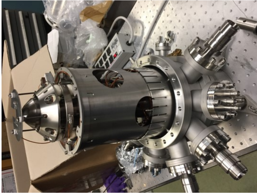
Figure 8.1: A photo of electron optics of the k-mic column. The TOF spectrometer is not included in this photo.
